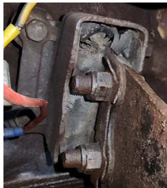
Driver's side motor mount before replacement
