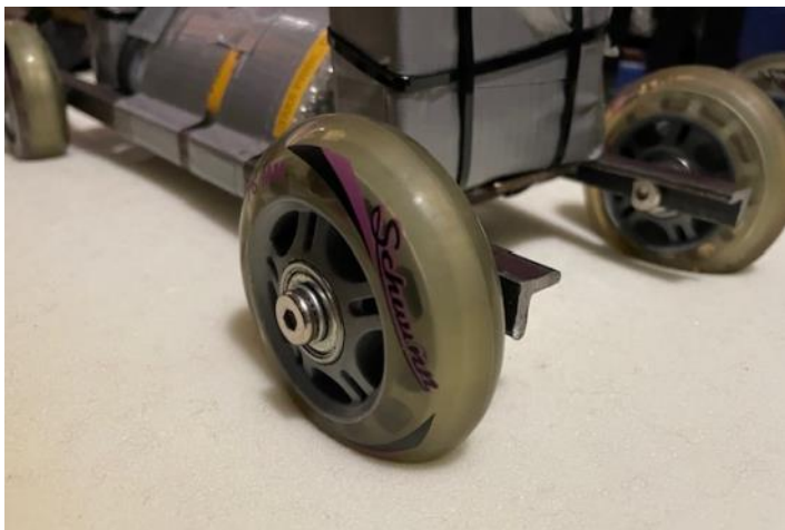
Wheel attachments must be solid and straight.
