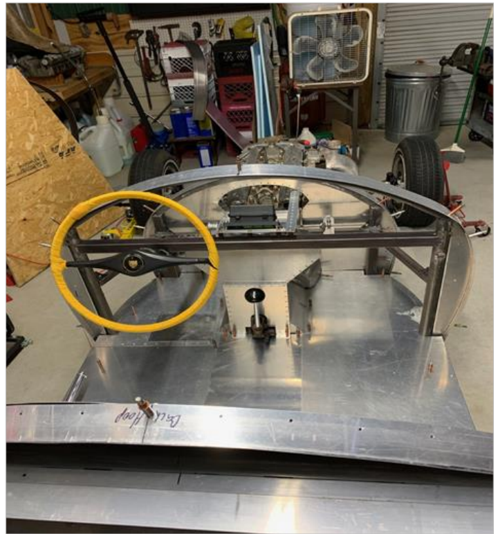
Here's a pic of the floor pan and trans tunnel, which is being held together with Clico clips until it's time for final riveting. I left the shifter mechanism exposed, to display the unique design of it in action.
