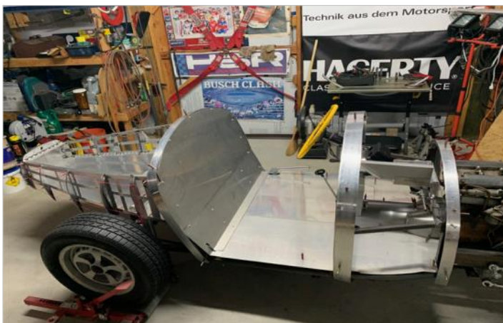
Side view of the basic body framing. Note the side ribs on the back boat-tail portion: each rib was formed with a different wood buck as the ribs had to get smaller towards the rear
