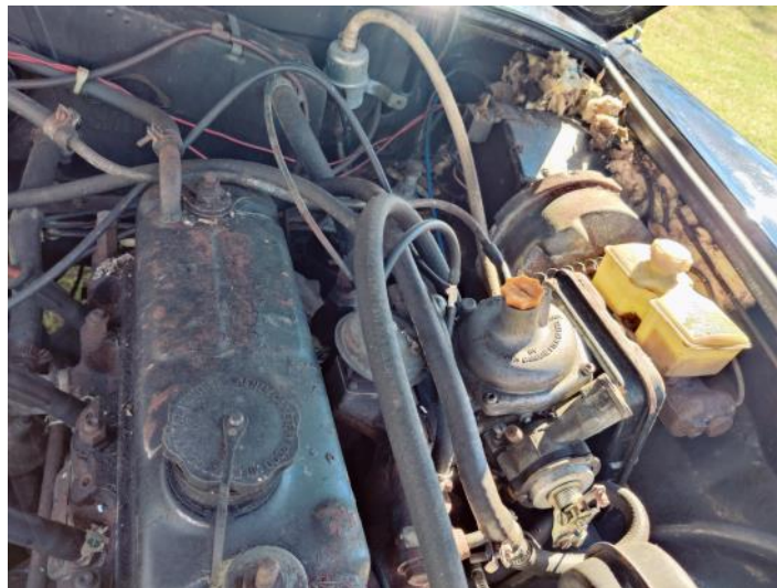
Evidence of rodent residency beneath the bonnet.
