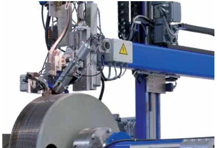
Automated welding head
