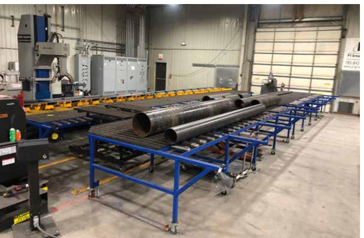
Pipe sections sit on a table as they wait to be loaded onto the pipe cutting machine. With the new pipe processing system, P1 Group fabricators aren't using as many heavy-duty carts to wheel pipe sections through the shop.
