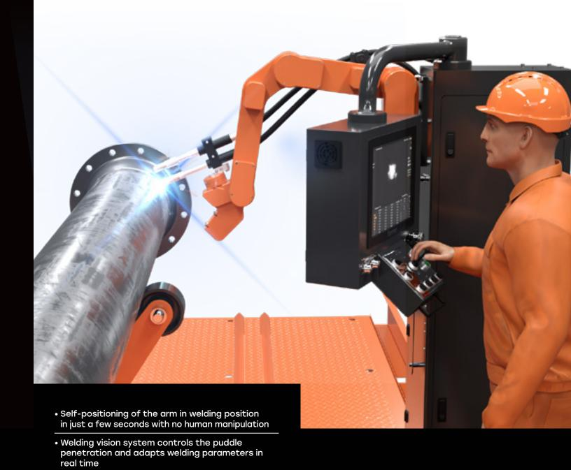
Embedded LED lighting allows the welder to easily align the torch in the bevel before starting to weld.
