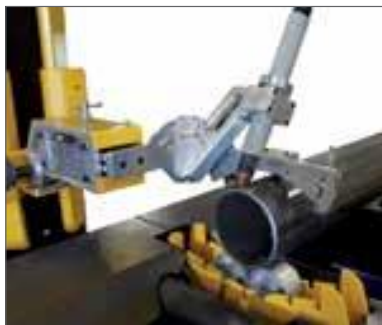
Watts W-122 - 2 CNC axes for round pipes with a maximum diameter of 14 inches compatible with most plasma cutting systems, floating chuck and manual adjustable pipe support units.
