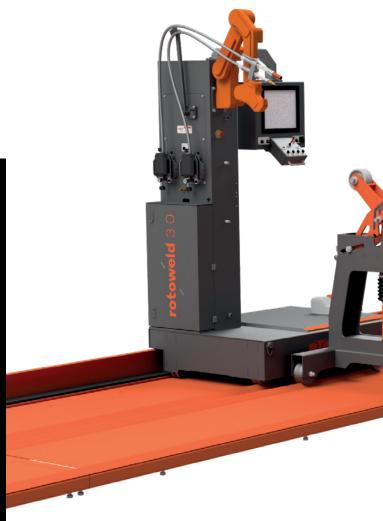
The Rotoweld 3.0 twin configurations include two separate work bays and rotators to maximize the work cell's throughput by allowing one work bay to be re-loaded while welding in the alternate one. The motorized welding carriage travels between work bays along a continuous track system, which also guides the idler rolls to maintain perfect alignment along the full length of the machine
