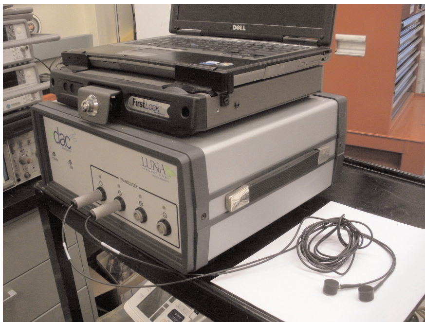
Figure 1 The pulsed phase locked loop (PPLL) device used to measure changes in intra-cranial pressure and corresponding changes in intra-cranial diameter.
