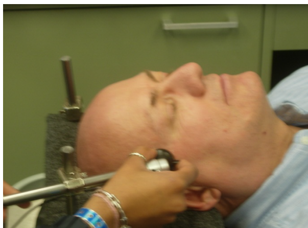
Figure 2 Transducer fixation system for tests conducted with the transducer placed over the temporal lobe.
