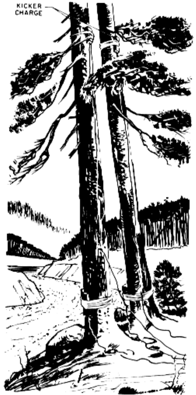
Figure 5 External and Kicker Charge Placement
