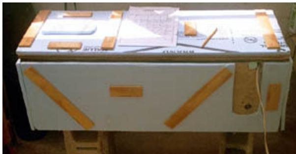
I cut up some plywood to make this box with a removable lid, covered the box with blue half inch insulation foam sheathing. The pieces of plywood nailed to the sheathing serve to hold the sheathing in place.
