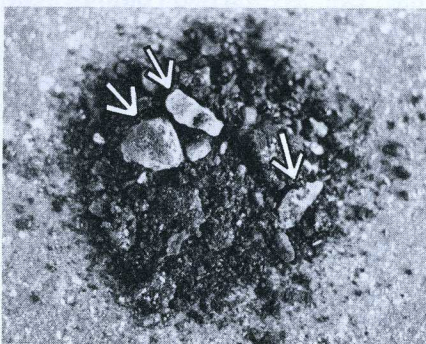
Figure 1-4. Arrows indicate deteriorated mortar that has come loose with the creosote during routine chimney cleaning. This is a sure sign of chimney problems.
