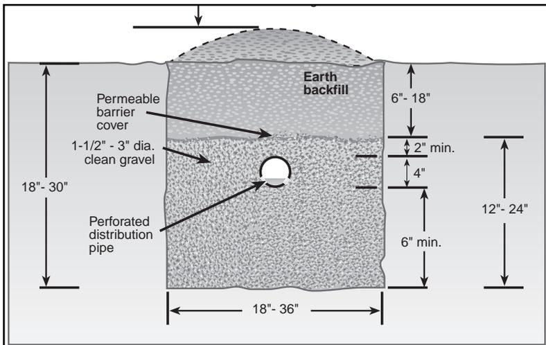
Figure 10. Section view of an absorption trench.
