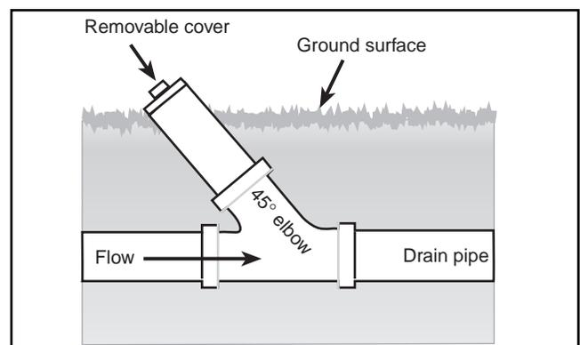
**Figure 3b. PVC pipe cleanout for drain pipe.**
