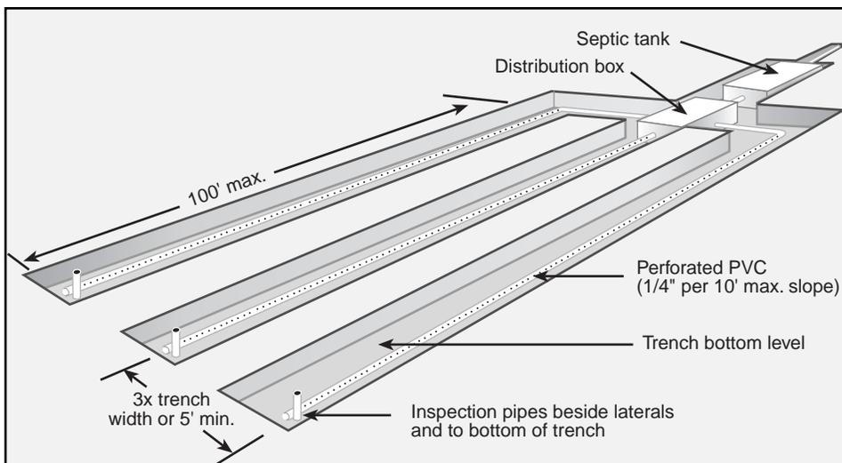
Figure 4. View of a typical absorption trench field.
