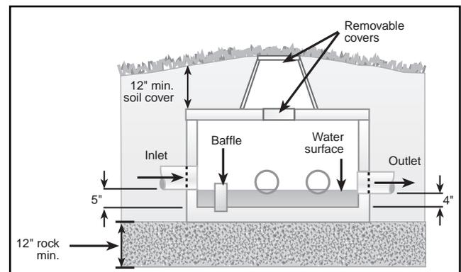
Figure 7. Section view of a distribution box, or D-box.
