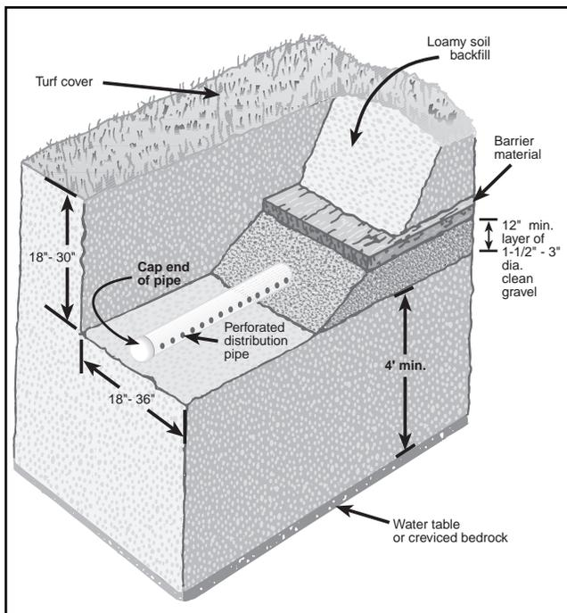
Figure 6. View of typical trench construction dimensions.
