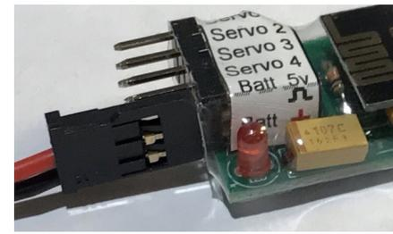
Connecting the power lead - red to centre, black (or brown) nearest to PCB. Note that Incorrect connection will damage the receiver. The spare pin can be used for telemetry feedback to handset. (Horizontal pins shown)
