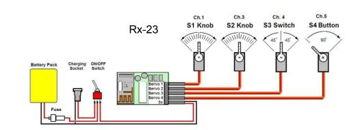
Rx-23 receiver circuit diagram for use with four Servos.
