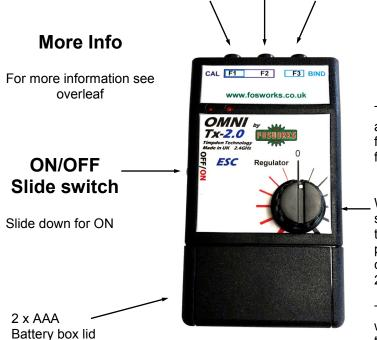
If Alkaline batteries are used up to 200 hours
