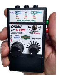
Regulator Knob full range control with Reverser switch to change direction.
