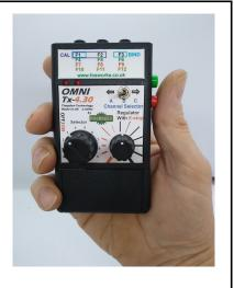
Regulator Knob Forwards and backwards with centre stop Selector switch allows three channels to be selected with 10 models on each of them selected using the selector knob.
