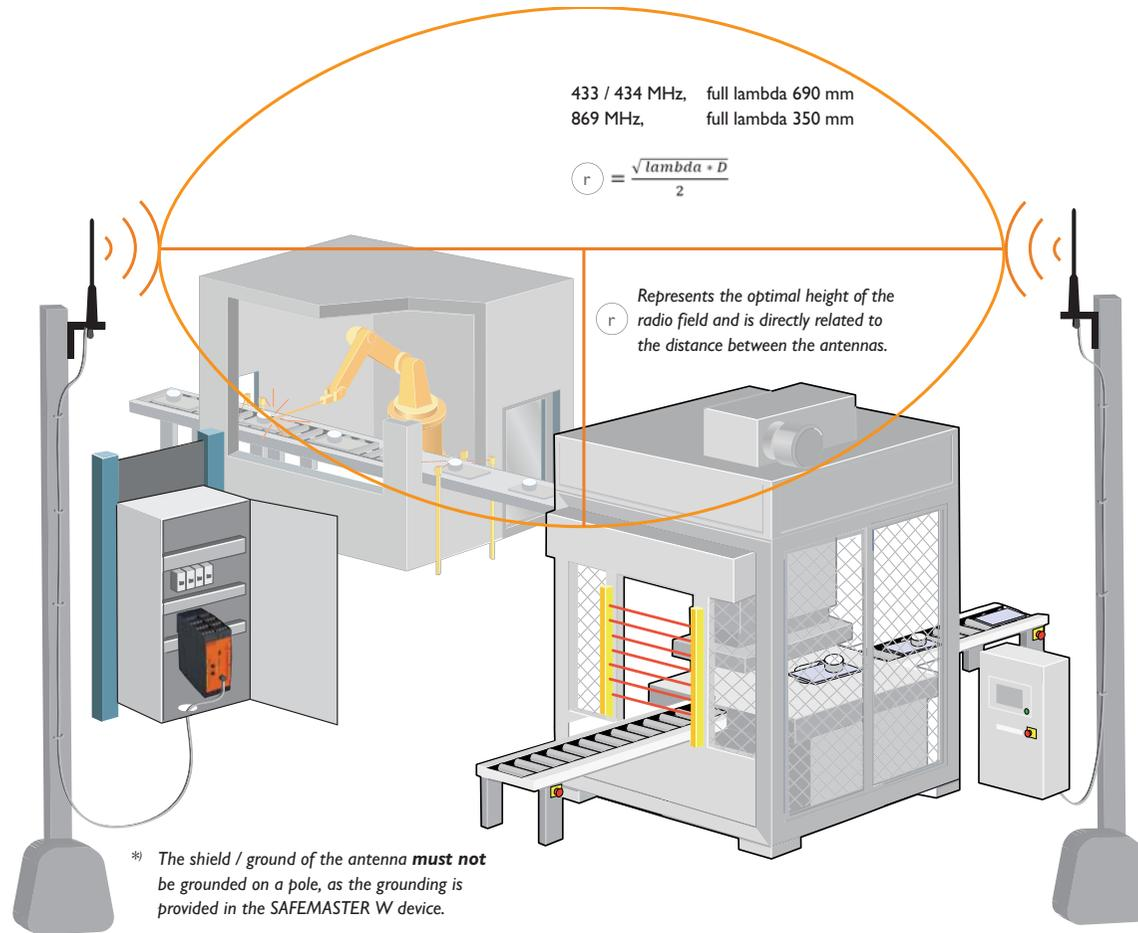
$r$  Is the optimal height differential of the antennas, two antennas should be installed within this height differential if possible. This is only advisory and may have to be altered with regards to ground clutter noise and reflections.
