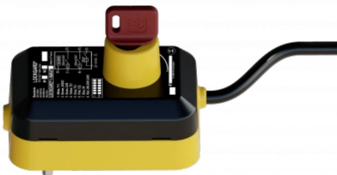
LOCKGARD M2.SP is an RFID key-operated safety switch with a key blocking device that allows : - the protection of an operator in a hazardous area by lockout. - the authorization of the energization of a dangerous machine The LOCKGARD® M2.SP RFID key interlock provides the complete PL e Cat. 4 safety chain according to ISO13849-1 when connected to an AWAX series enclosure. The LOCKGARD® uses an innovative principle offering control with a unique 16 million code RFID key.
