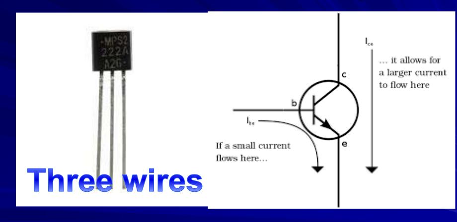
If a small current flows here, it allows for a larger current to flow here
