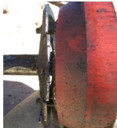
Figure 15 –Gauge plate with damage
