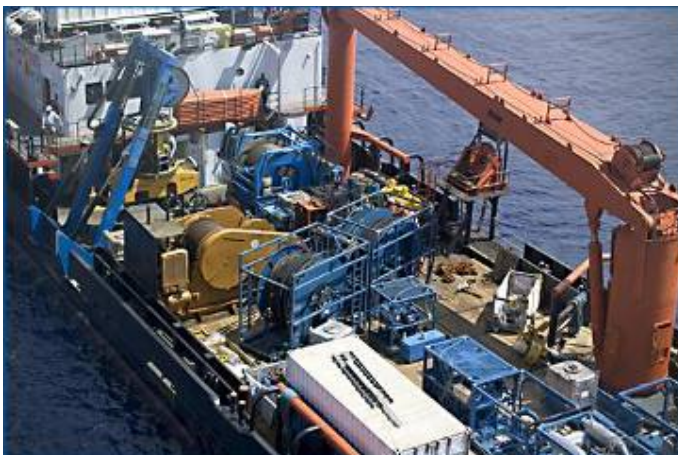
Figure 5 – on LHS shows a typical offshore vessel based spread required to deliver the above services to a subsea pipeline.
