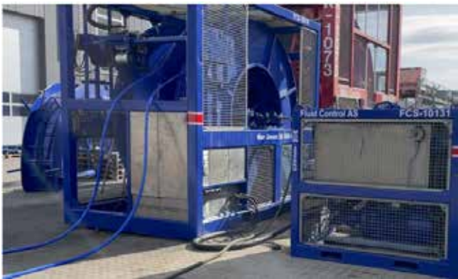
Figure 2. Powered hose reel with EnerMech twin composite downlines installed.
