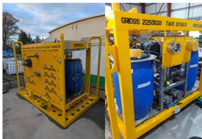
Figure 1. EnerMech Twin-Pump Umbilical STP Unit Front & Rear View (showing twin fluids).
