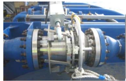
Fig. 15: Breakaway Coupling Detail
