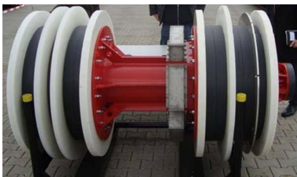
Figs. 16 and 17: Flooding, Cleaning and Gauging Pigs
