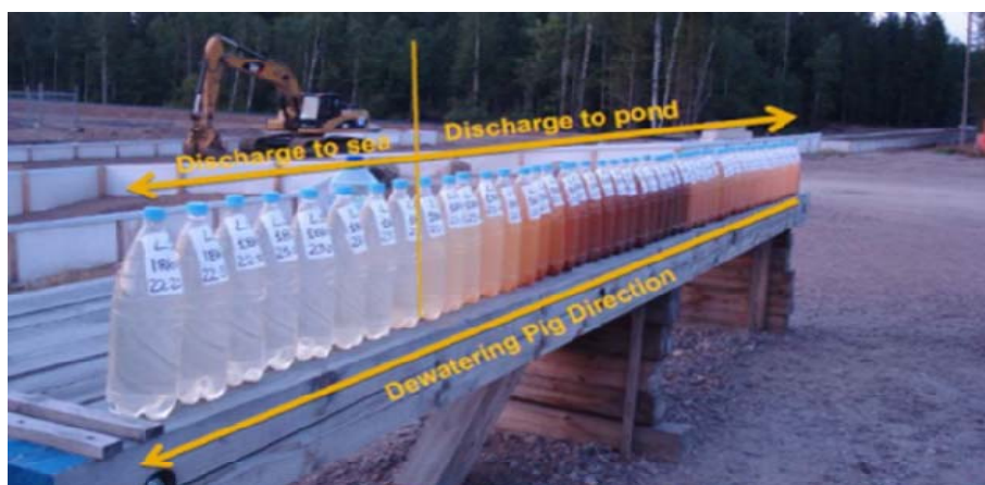
Fig. 28: Water sampling during dewatering train receipt
