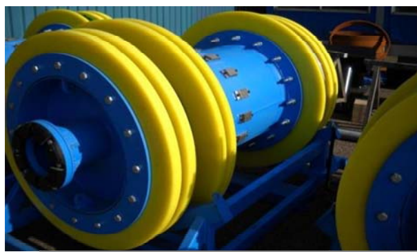
Figs. 16 and 17: Flooding, Cleaning and Gauging Pigs
