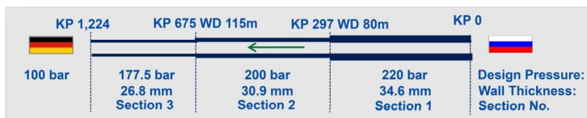
Fig. 2: Nord Stream pipeline segmentation
