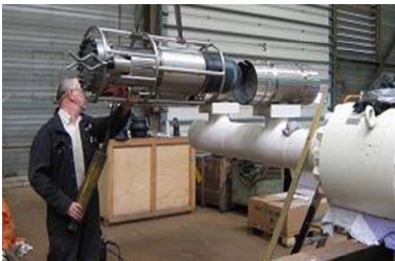
Fig. 12: 8-inch Low-Pressure Hot stab
