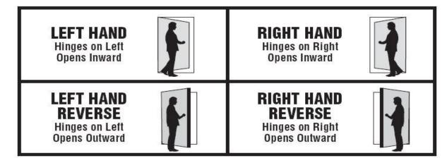
Stand on the secure side of the door (where you would insert your key). For pairs, determine the hand of the active leaf. The active leaf is typically the door with the lockset. Both leaves may be active.
