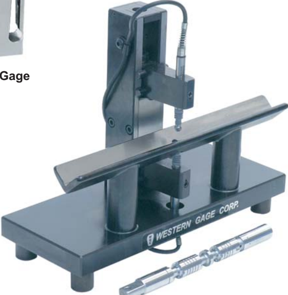
Vee Gage checks hydraulic valve spool O.D.s utilizing opposed set of LVDT Probes.
