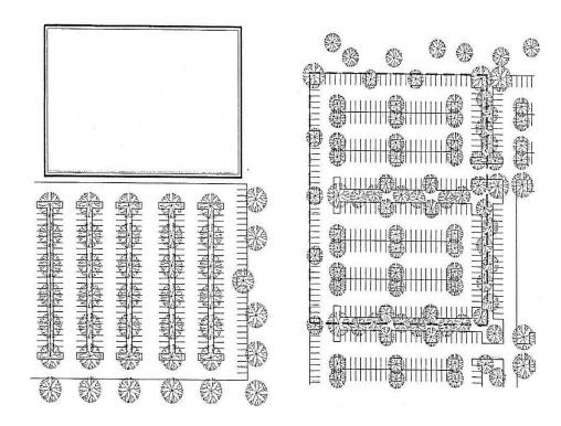
All parking lots should strive to incorporate LID components such as bio-swales and rain gardens to infiltrate surface water. The applicant is encouraged to provide interconnection between such features to maximize efficiency. (see Section 4-05.12).
