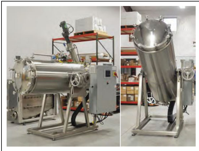
Figure 1. Bio-Response Solutions, Inc. Human-28 Low-Temperature Alkaline Hydrolysis System. The multistage process is carried out in a stainless-steel vessel with measured parameters including a specified alkali molarity, water-to-tissue ratio, rate of solution circulation, temperature, and operating time. A mesh basket is inserted into the vessel to hold the animal carcass. (Left) The mechanical control box is located on the far right. (Right) The vessel containing a mixing paddle is tilted into the operating position.
