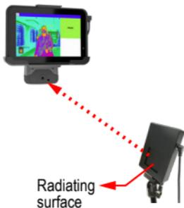
The radiating surface of the black body must face the camera's irradiation direction.
