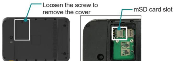
5. Follow the direction of the arrow to open the lid of the microSD slot.
