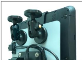
3. Mount the assembly to a metal surface. Please use it on flat metal surface.
