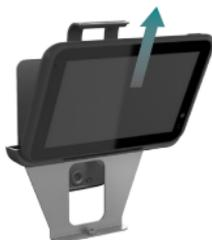
4. On the rear side of the HMI, loosen the screw to remove the expansion slot cover. Then you can see the microSD card slot.
