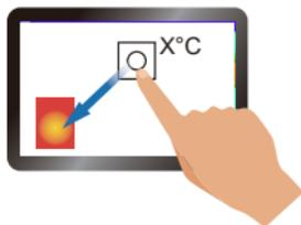
To further ensure the accuracy, use a forehead thermometer to measure one's temperature and see if MTA-3078T's gets the same measurement. If not, proceed to take the steps below to adjust the temperature offset.
