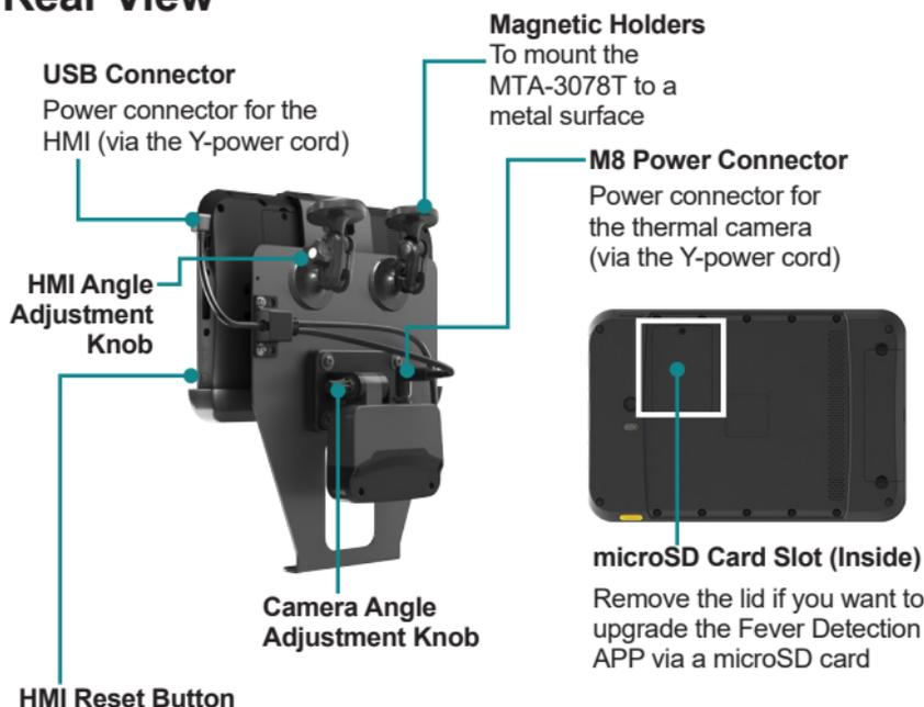
When the MTA-3078T is connected to power, press the **Reset** button and a power menu will appear on the screen. But the device will always reset itself when power is applied to the MTA-3078T.
