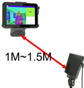
Place the blackbody at a distance of 1M~1.5M to the thermal camera.
