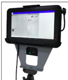
3. Adjust the height of the tripod and the tilt angle of the camera to ensure the blackbody and person to be detected are in the camera's field of view.
