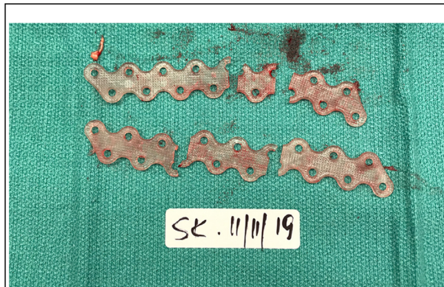
FIGURE 3 Explanted heavily fragmented BioBridge plates. Note lack of any resorption at 6 months, indicated by preserved surface texturing.
