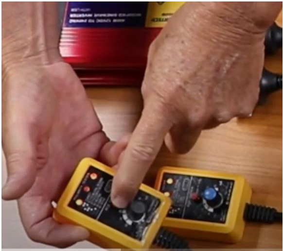
Images of existing PSOA and the WWEST PSOA showing Polarity test results
