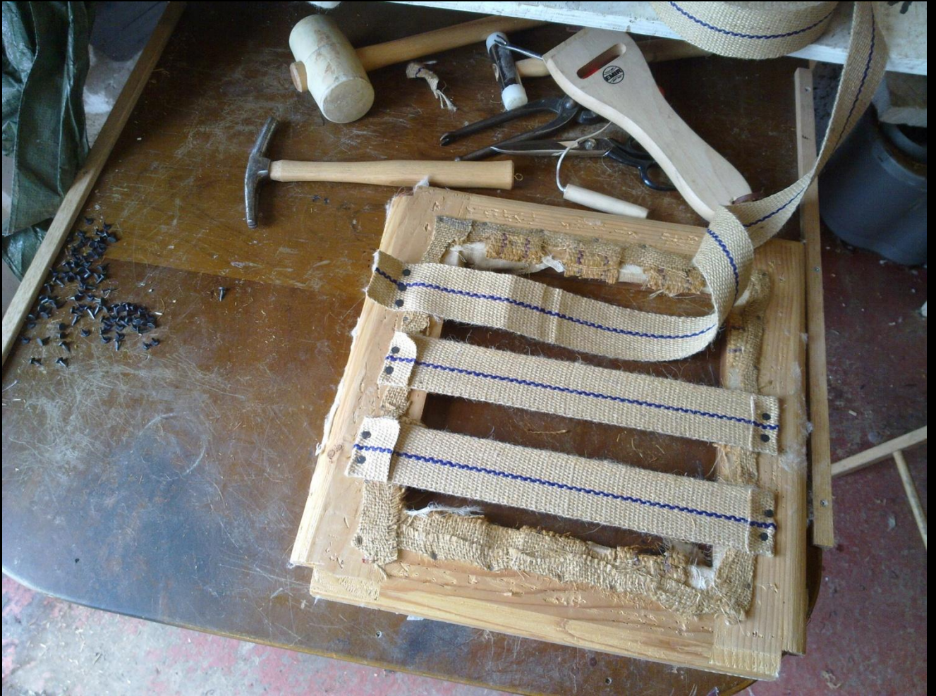
12lb jute webbing was tacked to the frame using 13mm improved tacks.
