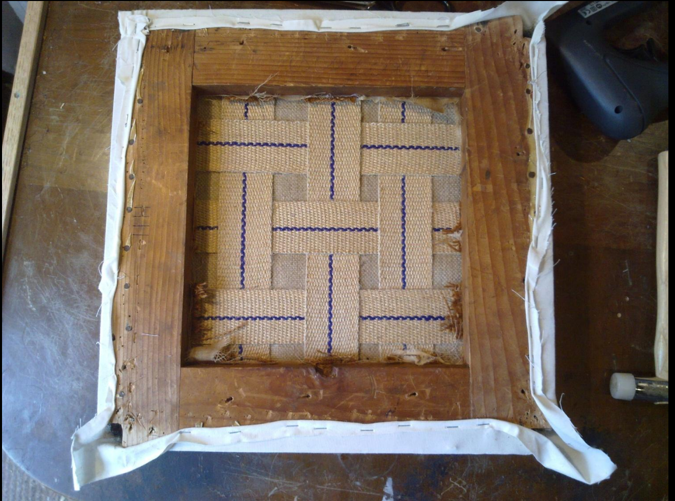
The fire retardant calico interliner is now attached, again using 8mm staples.
