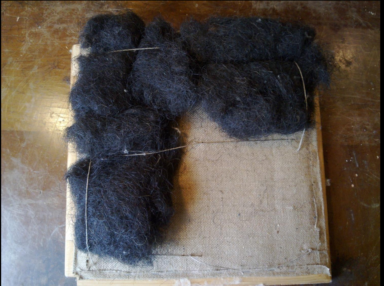
Linen mattress twine used to create stuffing. Horsehair then used to stuff the stuffing ties, teased out to ensure an even covering.
