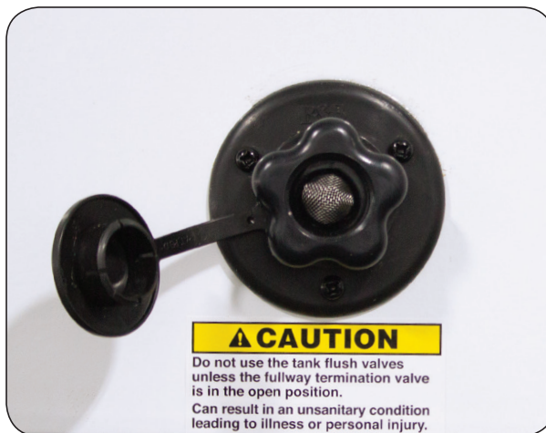
Black Tank Flusher Inlet is located on the off-door side of the RV.
