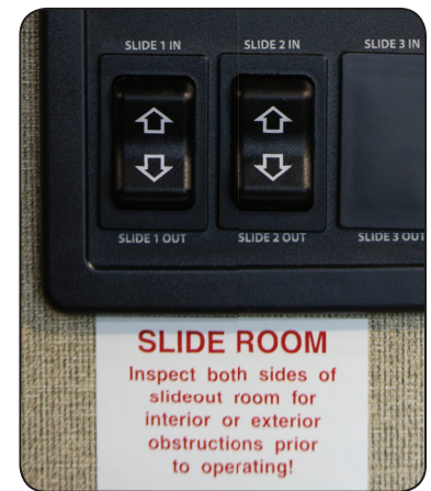
The Slide Room Switches are located inside the RV, on the Command Center.
