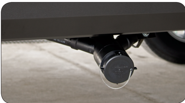
The Sewer Outlet Connection is located under the RV, on the off-door side.
