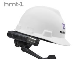
The RealWear HMT-1™ is a powerful, fully rugged Android computer that is worn on the head and replaces the touch screen with an articulated microdisplay to simulate a 7-inch tablet screen.
