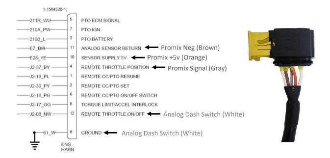
Pin 4 in remote throttle connector on firewall is the signal (0.5 min -4.5v max)
