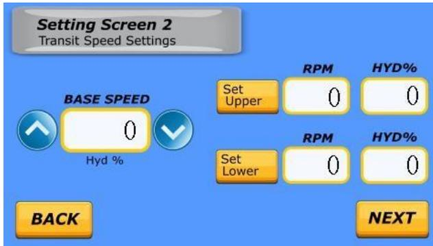
Base Travel Speed is controlled by the BASE SPEED setting. This is the percentage of hydraulic pump stroke during Travel Mode and has a range of 0-100%. Increasing this value will increase the base Travel bowl speed.
