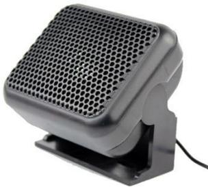
The external speaker should have a 4-8 Ohm nominal impedance and be terminated in a 3.5mm mono plug. When the external speaker is plugged in the internal speaker will be disconnected. (See page 14 for speaker port connection location)
