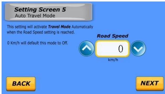
Travel Mode may be set to automatically activate at a preset road speed. The **ROAD SPEED** parameter value sets the preset speed in Km/h.
