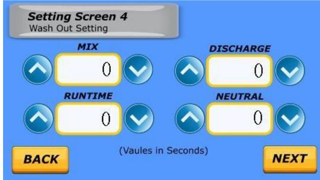
The Washout function parameters can be adjusted on this screen.
