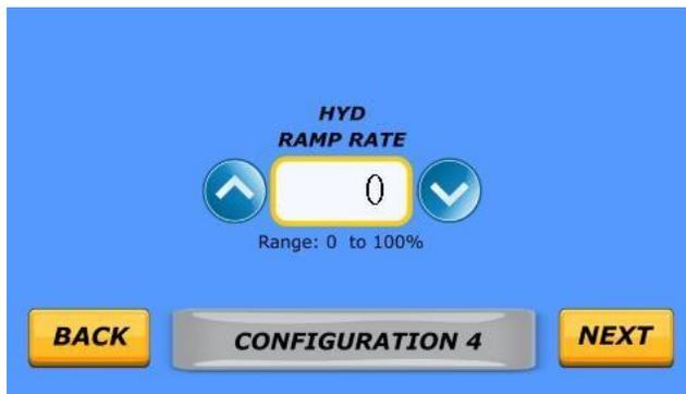
Hydraulic ramp rate is the time it takes for the hydraulic pump stroke to increase (or decrease) speed between minimum and maximum. The higher the value the faster the pump will ramp. Setting a value at or near 100% is very fast and may be dangerous. Use extreme caution when adjusting this setting.
