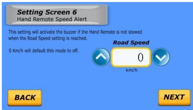
The Hand Remote Speed Alert may be set to automatically activate the visual and audible warnings at a preset road speed when the remote-control hand piece is not in the charging cradle. The ROAD SPEED parameter value sets the preset speed in Km/h.
