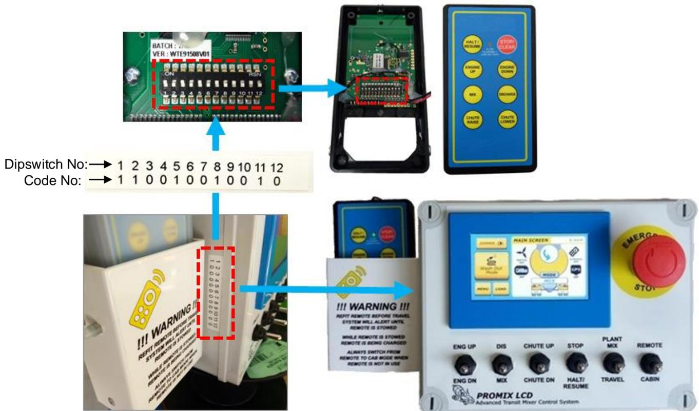
The hand held remote control transmitter contains a 12way dipswitch. In order for your transmitter to work with your console the code of the 12way dipswitch must match the code on the label beside the charging cradle (see image above). A “1” indicates the corresponding switch should be in the “ON” position. A “0” indicates the corresponding switch should be in the “OFF” position.
