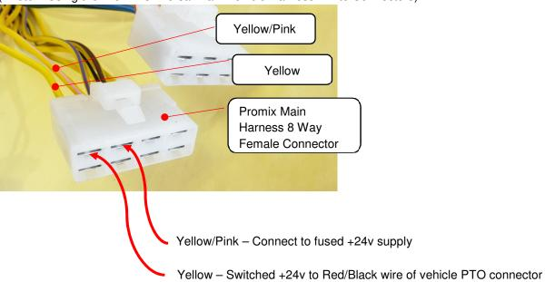
Relay contacts within the Promix console join the Yellow/Pink and Yellow wires when analog revs control is selected and appropriate lockouts are active. Maximum load for this circuit must be below 60w.
