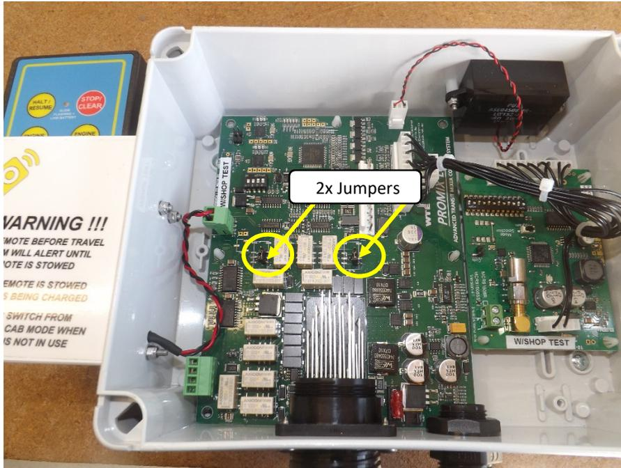
Electronic Hydraulic Pump Selection must now be made with both the on-screen menu and two physical jumpers on the PCB.
