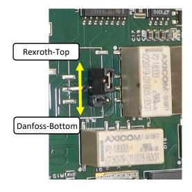
For Rexroth, both jumpers must be in the TOP position.
