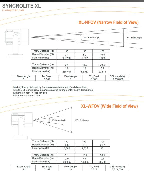
Multiply throw distance by Tn to calculate beam and field diameters. Divide CBI (candela) by distance squared to find center beam illuminance. Distance in feet -> foot candles
