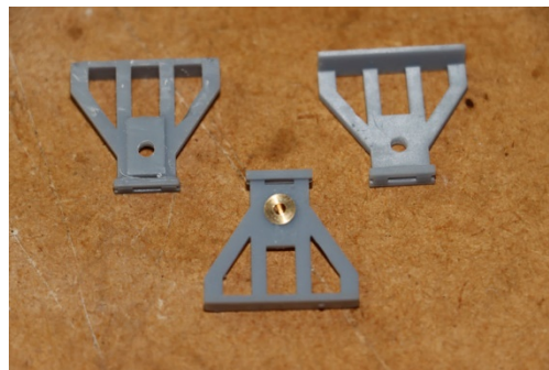
Figure 1 Axle guard with Slaters bearing.
