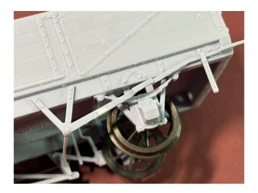
One end of the long cross bar fits into the single V hanger. Onto the other side the cross bar passes through the brake print containing the brake shoes, link rods and actuator.
