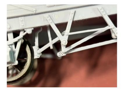
The other end of the drive link uses the short bar to connect the drive link to the right hand V hanger.
