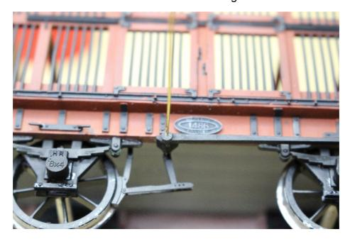
Thread the brake lever guide on to the brake lever – its easier to insert with the brake guide 90 degrees out then rotate the brake lever guide to the correct orientation.
