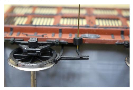
Thread the brake lever on to the wire – the bass facing outwards.
