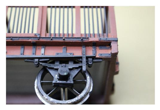
Adjust the position of the brake lever guide to the correct position and sitting vertical, then glue in place.
