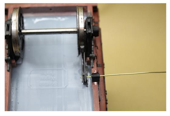
Feed the wire a few millimetres past the inner edge of the brake shoe, apply a spot of glue the wire both between the shoe assembly and the pivot block and to the inside of the shoe.
