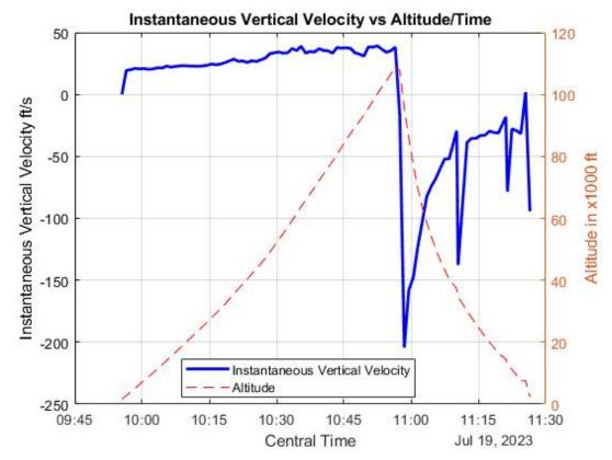
During the approximately 90-minute flight, the sounding balloon reached a maximum upward vertical velocity of approximately 40 feet per second, and a maximum downward vertical velocity of 205 feet per second after the balloon's controlled explosion.
