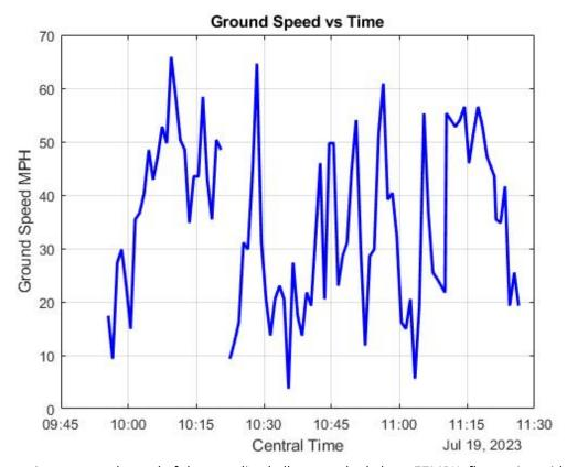
The maximum ground speed of the sounding balloon reached about 77MPH, fluctuating with the wind speed.
