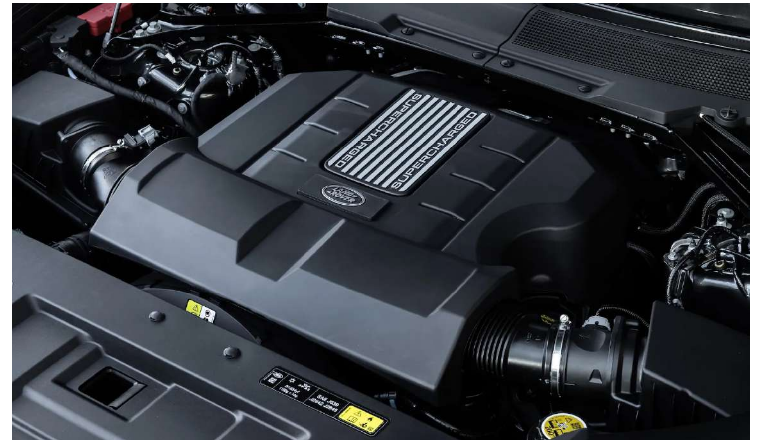
5.0L Supercharged V8 - 518 HP
