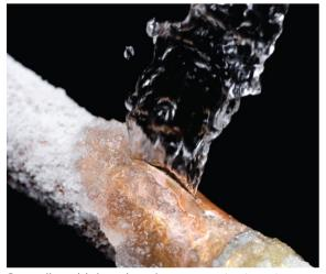
On really cold days, keeping your water tap at a trickle can help pipes from freezing and bursting.
