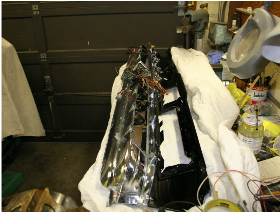
Dash rear before instruments were installed
