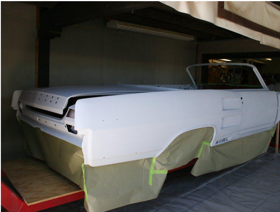
Body primed after finish of rear parts on body
