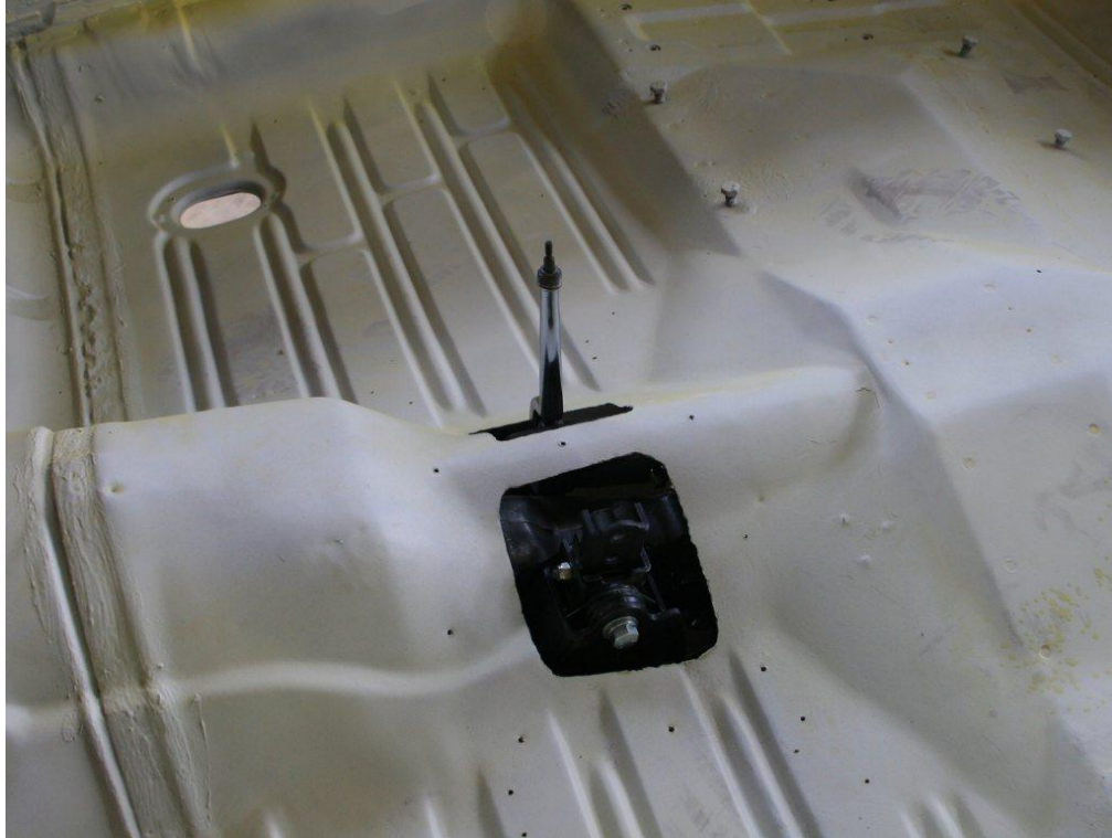
Exhaust cutout control lever appearing through the floor hole.
