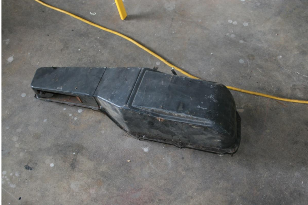
Heater box stripped of paint
