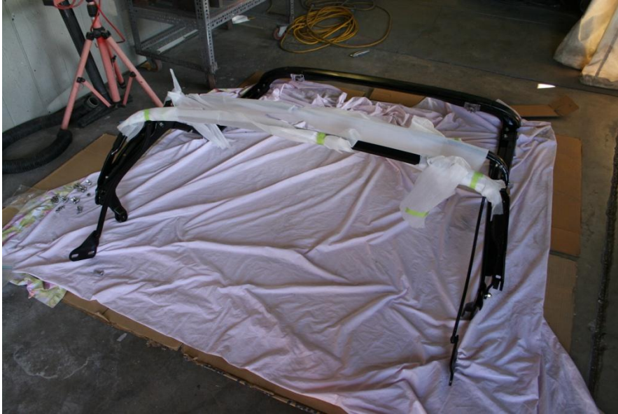
Top bows assembled and ready for installation
