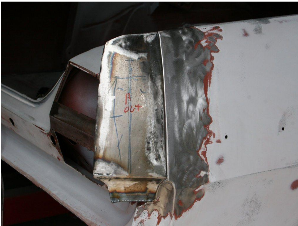
Fit up of the part on the back end of the body
