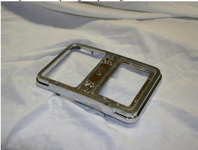
Shifter plate with hole for exhaust cutout lever
