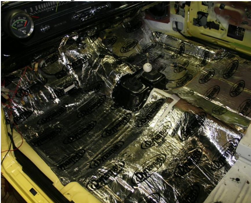
Sound deadener installed
