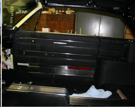
Finished panel installed on door
