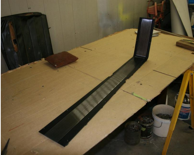
Rear console plate. Solid brass plate machined for console
