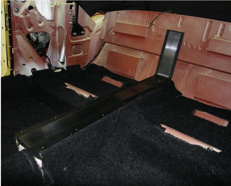
Rear console fitting and carpet installation
