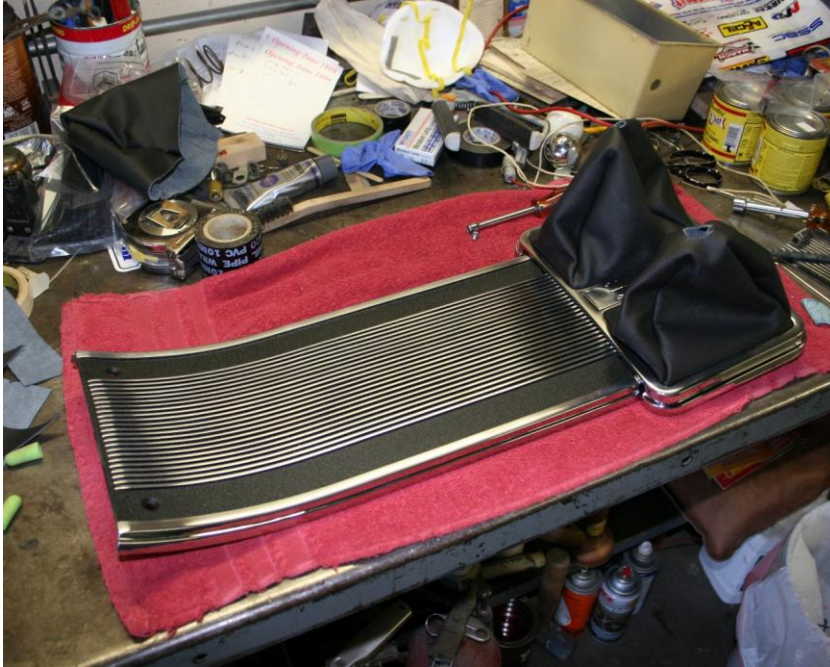
Shifter boots installed on the floor plates
