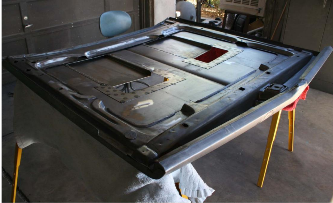
Back side of hood with brace removed
