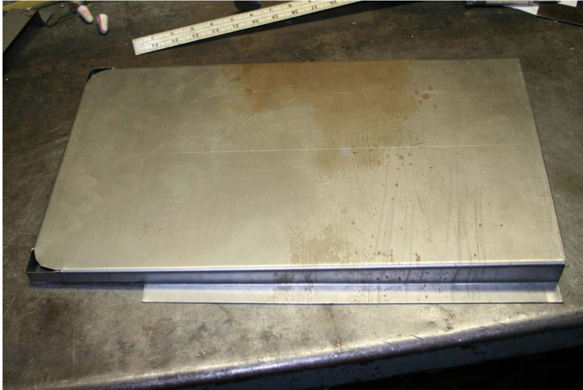
Hood scoop being formed
