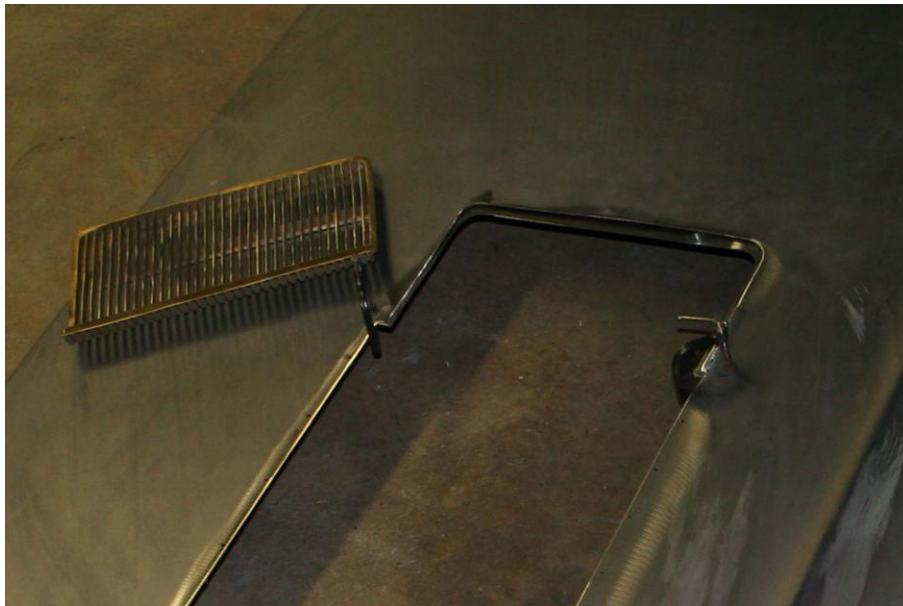
Metal supports being attached to hood
